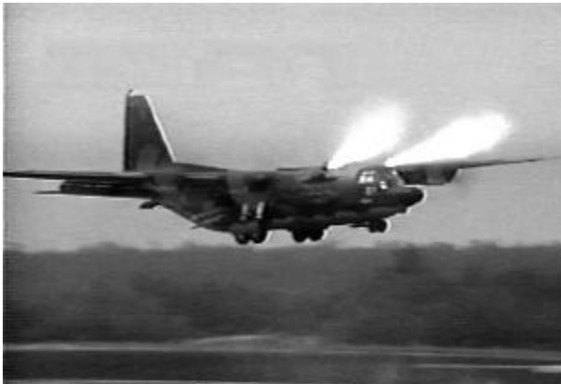
USAF Photo Aircraft 74-1683 begins its rocket-assisted maximum-effort landing. The top four reverse-mounted ASROC rockets have fired to slow the aircraft's forward flight vector.
