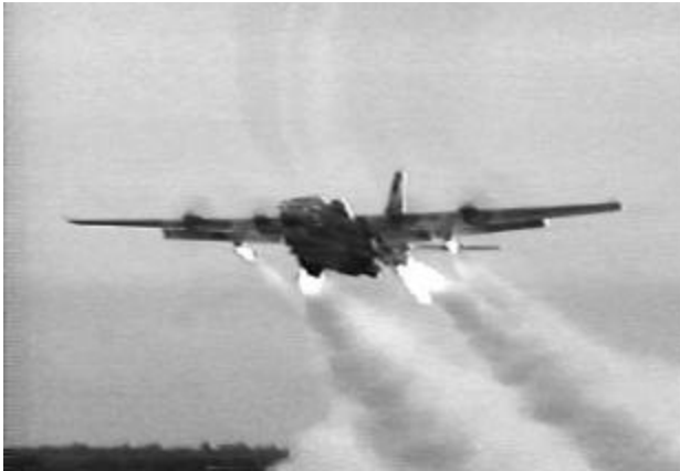
USAF Photo Credible Sport aircraft 74-1683 performs a rocket-assisted short-field takeoff on 29 October 1980. From brake release to liftoff, the aircraft traveled 150 feet.
