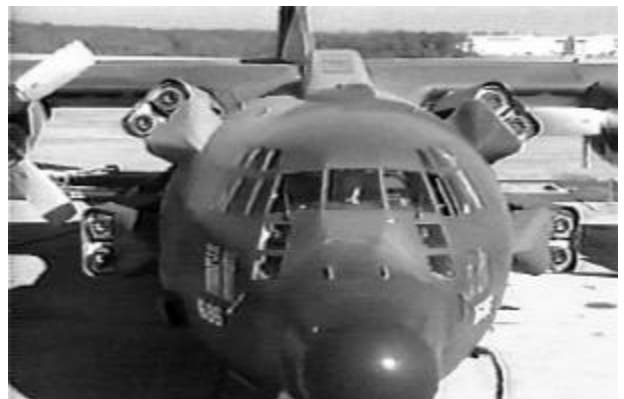
USAF Photo Front view of Credible Sport aircraft with eight ASROC rockets extended.
