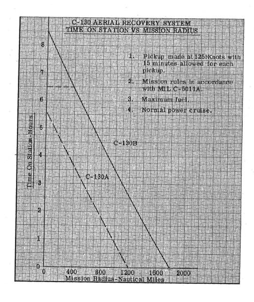
weight empty will vary with time-on-station inasmuch as the number of aerial pickups planned, which determine the required time-on-station, also determines the amount of equipment carried in the airplane.
