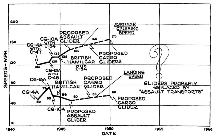
Figure 7-8 --- Performance Characteristics of Troop Carrier Gliders
