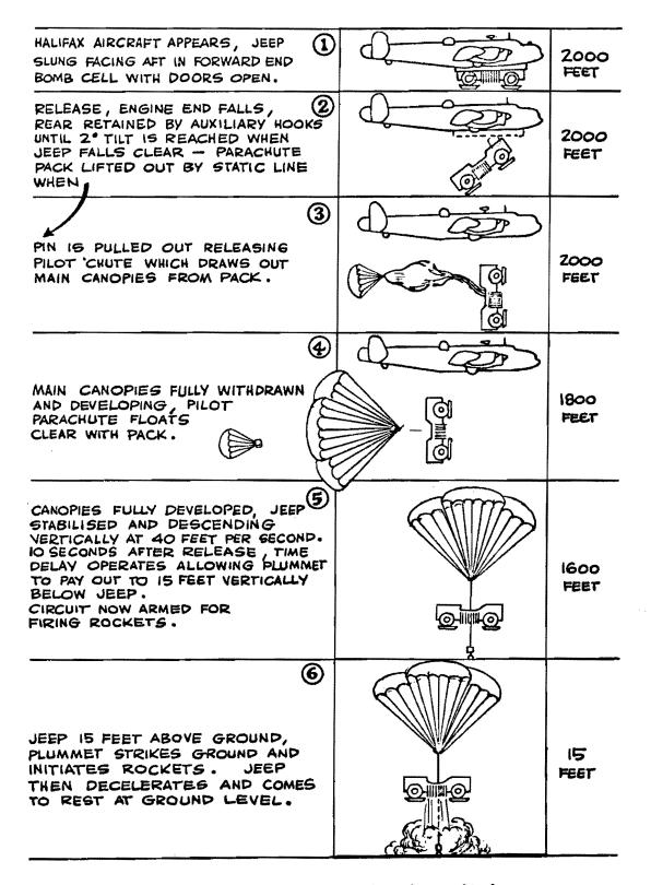
Figure 10 — Dropping a Jeep by Means of Parachutes and Rockets
