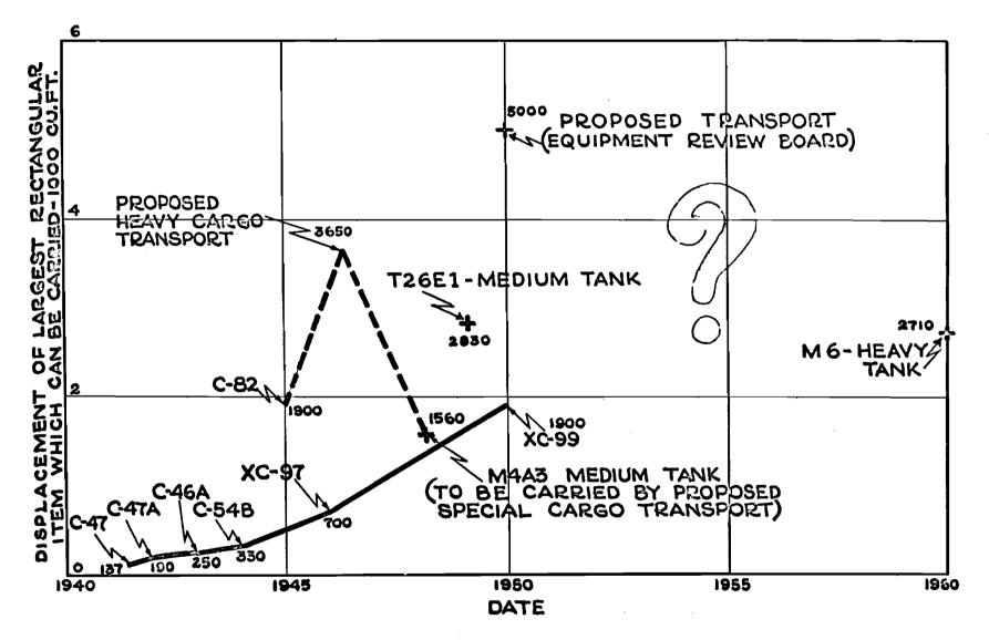
Figure 4-8 - Carrying Capacity of Troop Carrier Airplanes
