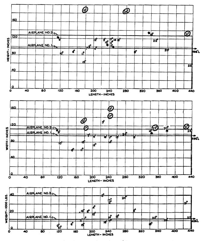
Figure 11-C — Weights and Dimensions of Army Equipment (Aviation Engineer Equipment)
