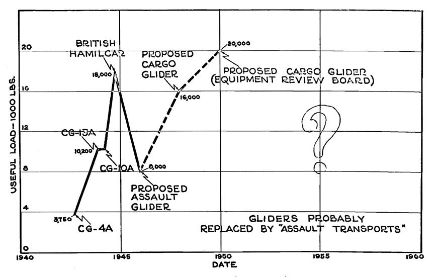
Figure 6-A --- Carrying Capacity of Troop Carrier Gliders
