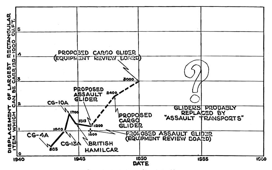
Figure 6-B ---- Carrying Capacity of Troop Carrier Gliders
