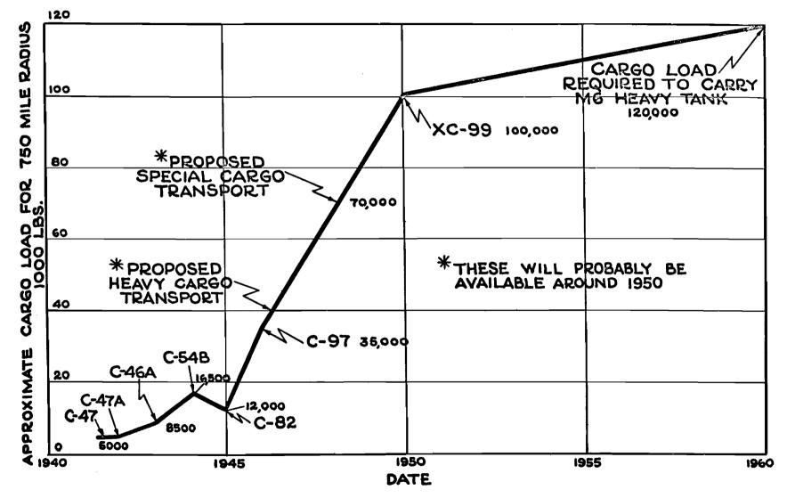
Figure 4-A — Carrying Capacity of Troop Carrier Airplanes
