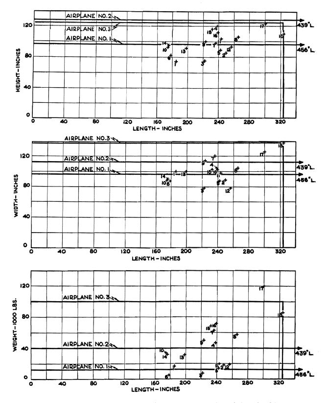
Figure 11-D — Weights and Dimensions of Army Equipment (Combat Vehicles and Tanks)
