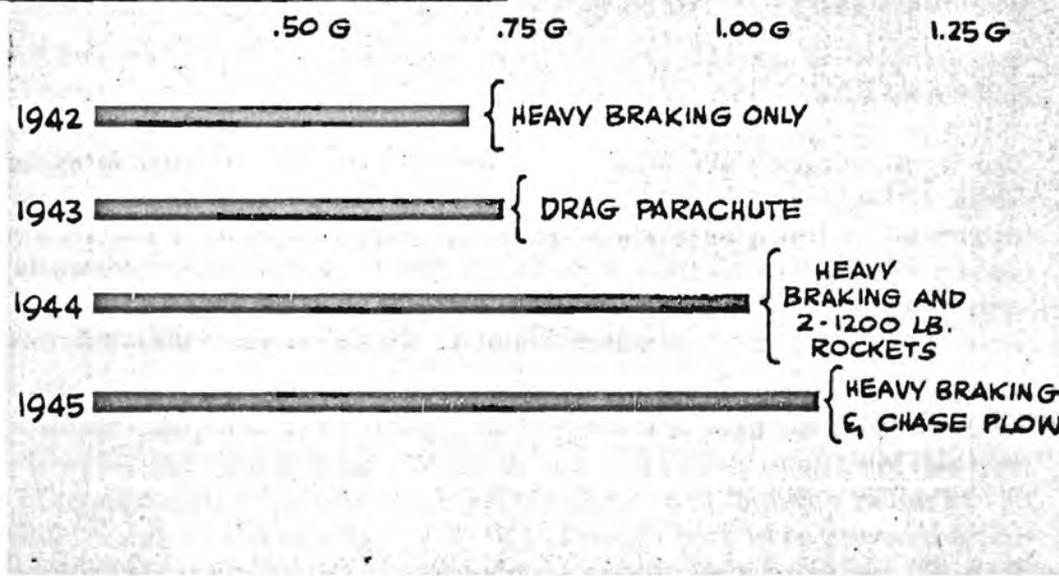
Figure 8 — CG-4A Glider Gross wt 7500 lb Landing Speed — 55 MPH
