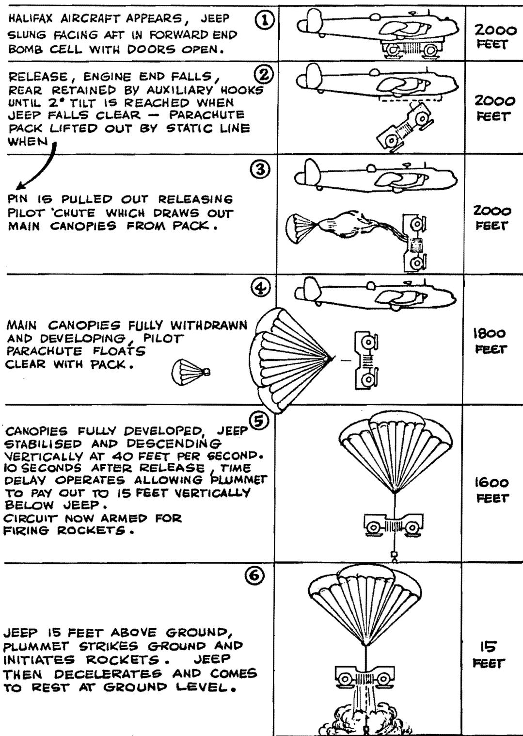
Figure 10 — Dropping a Jeep by Means of Parachutes and Rockets
