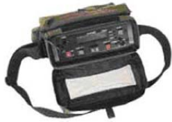
SARFIND (Search and Rescue Finder Decoder) reads and displays the location of the airdropped item(s)
